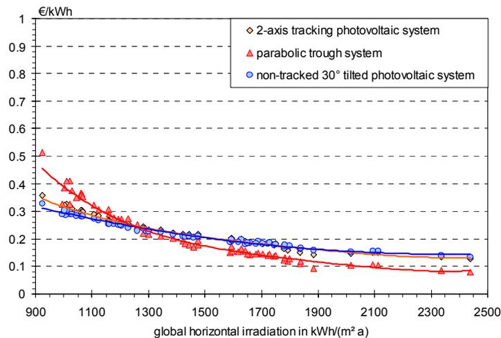
Figure 10. Levelised electricity generation costs in 10 years for photovoltaic systems and 1-axis tracked concentrated parabolic trough systems as function of the global horizontal irradiation
