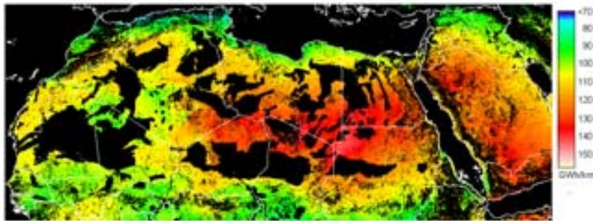
Figure 11. Annual Solar Electricity Yield of Solar Thermal Power Plants (200 MW<sub>c</sub> SEGs) in Northern Africa. The total potential of  $13 \cdot 10^6$  TWh<sub>e</sub>/year can theoretically cover about 1000 times the world electricity demand
