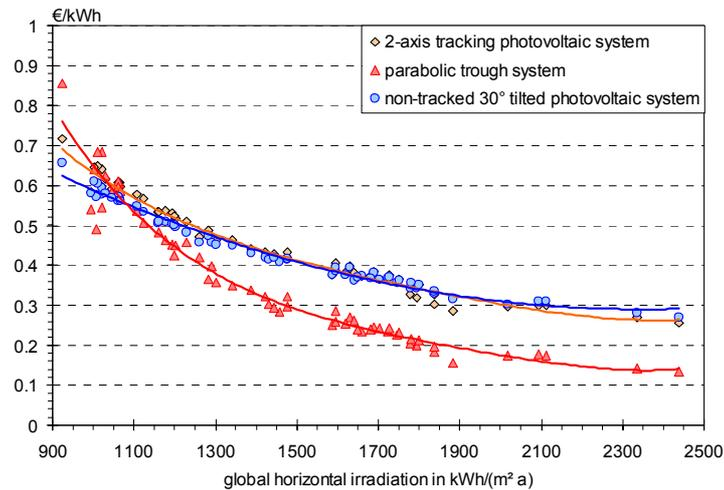
Figure 9. Today's Levelised electricity generation costs for photovoltaic systems and 1-axis tracked concentrated parabolic trough systems as function of the global horizontal irradiation
