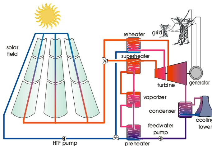
Figure 2. Principle of the parabolic trough power plant
