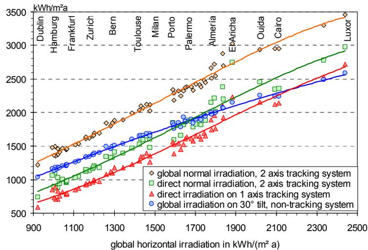
Figure 8. Direct normal irradiation, direct irradiation on a 1-axis tracked collector, global irradiation on a 30° tilted plane and global irradiation on a 2-axis tracked plane as function of the global horizontal irradiation
